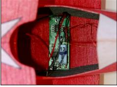
Place the RFFS-100 horizontally in the center of the cockpit. I gently pressed it into the bottom wing until the posts beneath the battery and motor connectors penetrated the wing. This keeps the board from sliding forward or back, and holding it down with a finger as you remove the battery leads keeps it from being pulled up. I use a length of thin coated copper wire for the antenna, which is passed to the rear of the fuselage and exits through a small hole in the bottom sheeting.
