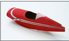
Carefully glue in the fuselage former F1, making sure it's straight and flush with the front edge of the fuselage. Next, glue together the rear-most edges of the fuselage halves together (where the rudder will eventually attach). Finally, glue in formers
