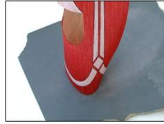
Sand the front of the fuselage to provide a completely flat surface for the cowl to mate with, then glue the cowl on. Also, reinforce the bottom opening (directly in front of where the bottom wing will attach) with some string saturated with CA. The wood is fairly stressed in this area, and could split without this reinforcement.
