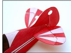
Connect the two elevator halves with a small 1/16 inch stick, then attach the elevator to the horizontal stabilizer with thin slivers of rubber band. Glue the horizontal and vertical stabilizer to the fuselage, making sure they're in alignment, then attach the rudder.
