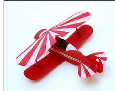
Attach the top wing by first gluing the interplane struts. These struts will set the correct position of the top wing, and you can then glue in the cabane struts, made from 1/16 inch sticks sanded round. Use the cabane struts to make sure the incidence angle remains constant across the top wing.
