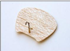
Before gluing in F2, create a small "J" hook from thin music wire, and attach it to F2 with length of rubber band. There should be 1/8 inch of rubber band between F2 and the hook. This will be used to secure the battery in the cowl. When gluing in F2, angle it to provide 6° of right and 3°
