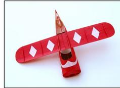
Attach the bottom wings by carefully sliding them through the slots in the fuselage and gluing them together. Once together, position and align the wings within the fuselage and glue with a small drop of CA on the leading and trailing edges on the inside of the fuselage.
